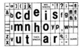
One of the cases in which printers kept their letters (metal type). The arrangement of the letters is based on frequency of use rather than alphabetical order. The most used letter is **e**.
