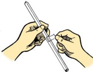
**To make the pipe:** roll one sheet of paper lengthways to form a tube. It should measure not more than 2 cm across the ends. Make sure that the ends of the tube are level. Then fasten the centre with a piece of sticky tape.
