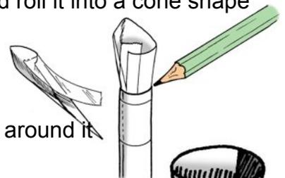
Put the cone into one end of the pipe and let it rest there. Draw a line around it where it meets the rim of the pipe.
